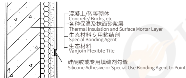
① 硅酮胶或专用填缝剂勾缝 Silicone Adhesive or Special Use Bonding Agent to Point
